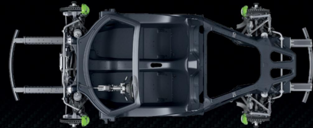
Monocoque and unit carrier
